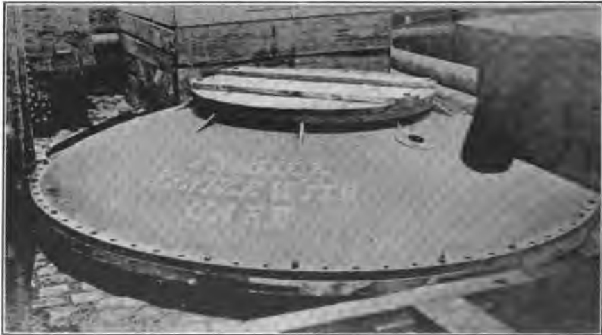
FIG. 138.—A cast-iron evaporator dome of 10 ft. diam. shipped from France and transhipped in New York to the West Indies: an example of careful packing.
